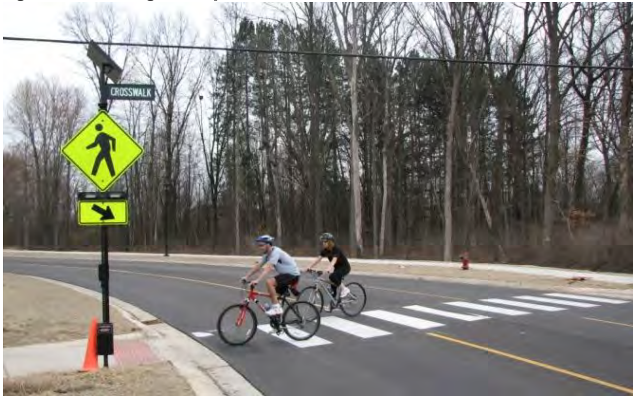
Fig. 9.7H. Rectangular Rapid Flash Beacon
